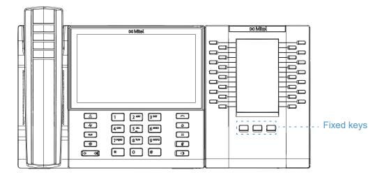
The M695 features a 4.3" 480x272 pixel color backlit LCD display.
