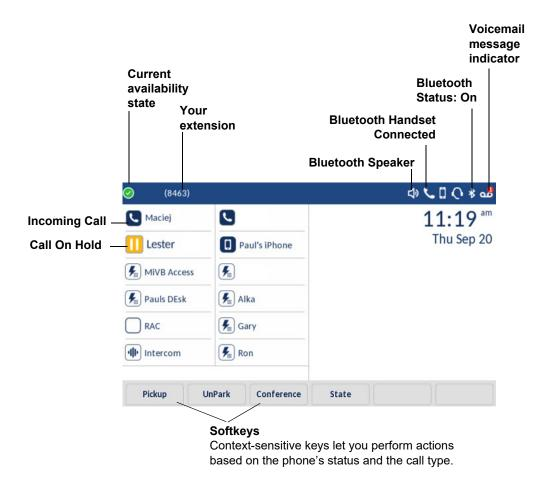
Figure 3: Elements on the Display Screen of the 6940 IP phone
